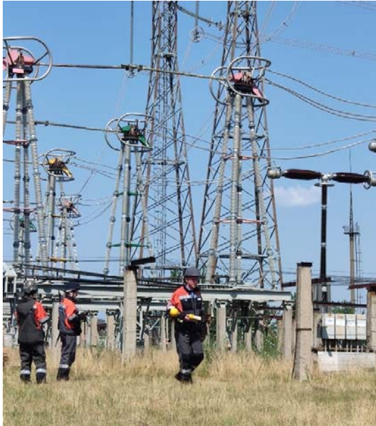
Figure 1. The example of electric and magnetic field measurement in open switchgear
